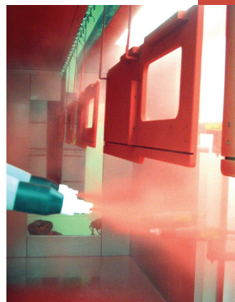
Parts are sprayed in a mist of powder, which is electrostatically attracted to the part.
