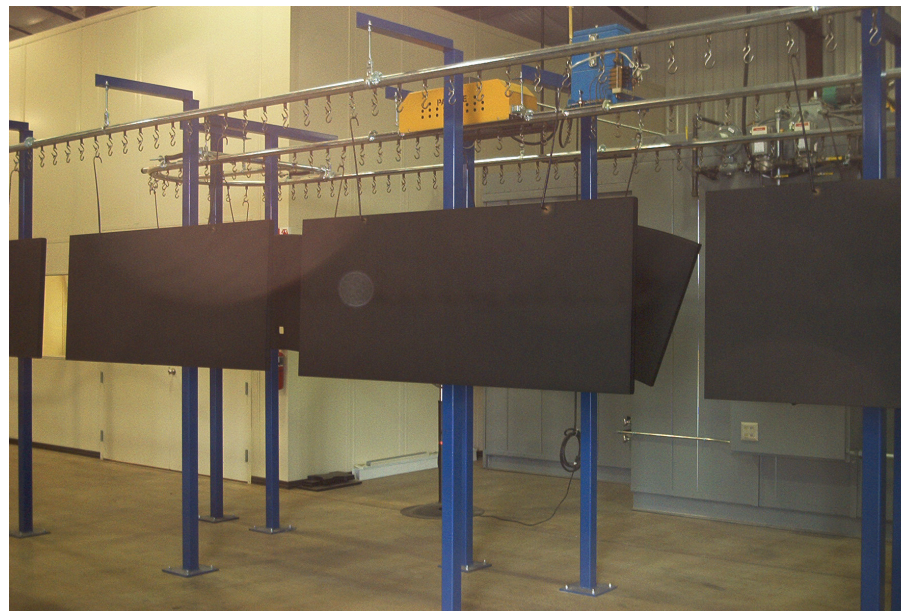
Large parts can be mass produced on a conveyor system.
